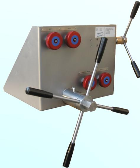
All tubing is made of stainless steel 316 and M16x1.5 or 9/16"x18 UNF high pressure connections are used.
